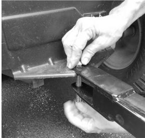
1 **The Model 65PT** is designed to spread compost, sand, and topdressing blends. The unit is available with two types of tongue - one to fit the drawbars of conventional, 4-wheel tractors and one to fit 2-wheel, walk-behind tractors. Attach tongue to drawbar using a threaded bolt and secure with a nut or with the proper hitch pin.
