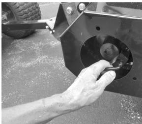
4 **To Begin Spreading**, engage the clutch pin on the left side of the machine. Adjust the endgate opening using the adjustment handle, (see Maintenance #6) so that it is open the right width for the spread depth desired.
